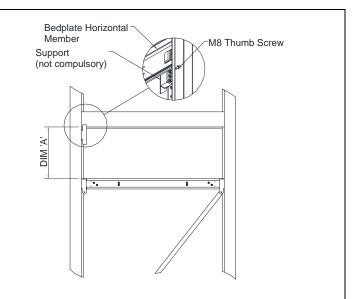
The cable chain is secured to a mounting bracket which spans two horizontal members. This should be positioned to mount the end of the cable chain at a position of half the travel plus 200mm above the pit floor.
